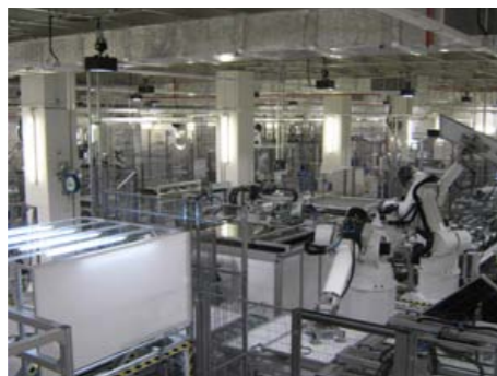
View of the fully automated framing range of a partial line.
