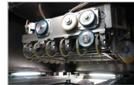
Bricking with Diamond Wire
